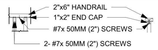
DETAILS (SB-7 DETAIL EC-1) END CAP AND PICKET ATTACHMENT, TYPICAL
